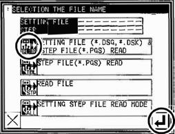
(4) The screen to select the step file is displayed. Please choose the [2008HT \* \* ] by using up and down arrow button. (The \* \* mark displays file version.)
