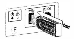
(3)While holding down the [F] key on the front panel of the control box, turn the machine power ON. (Keep pushing [F] key until red LED on the front panel is turned on.)
