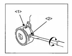
(2) Bobbin thread tension (Rotary hook type) Adjust the bobbin thread tension with the thread tension Adjusting screw (No.2) on the bobbin case (No.1). The thread tension become loose if turn the thread tension adjusting screw (No.2) to the counterclockwise, and the thread tension becomes tight if turn it to the clockwise.
